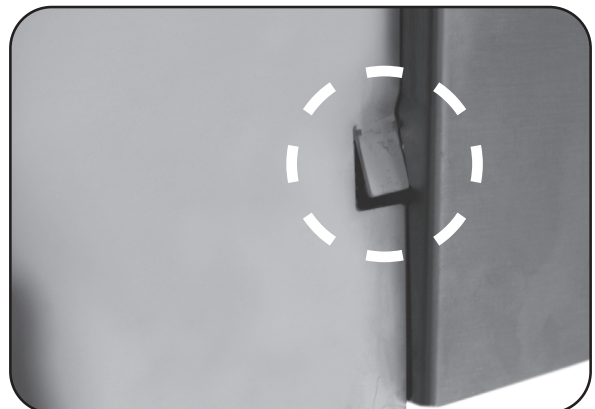
Fig. 19-4 Tab slightly bent in for clearance
